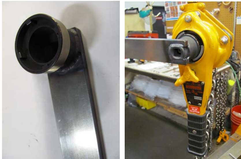
Figures 6 and 7: Adjusting slip clutch lock nut with adjustment tool vi. Return to step 2.b.
