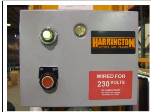
Fig. 6 – Tester Control Panel
