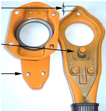
L5 Lever Redesigned and Material Thickness Increased
