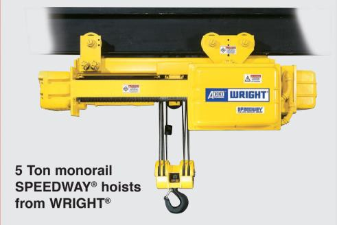
SPEEDWAY® hoists are an excellent choice for lower volume lifting with 30 minutes of operation per hour with a maximum of 300 starts an hour as defined by Hoist Duty Class H4 of ASME HST-4.
